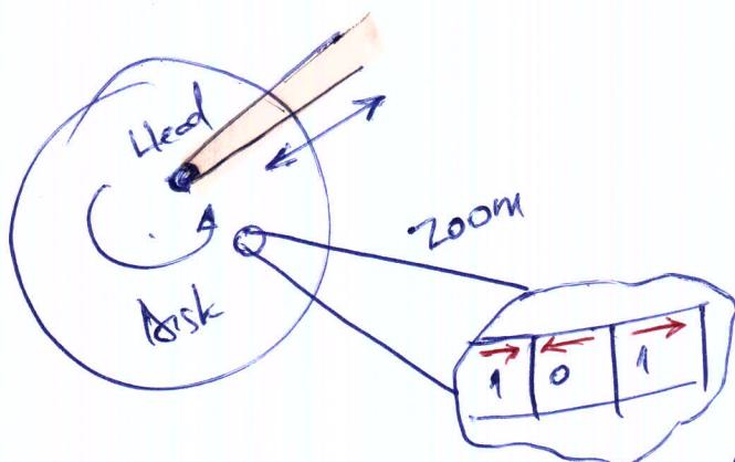
The head-coil feels changes of  $\Phi_B$  when passing domains (1) and (0) (B-vanes) which are translated "in emf"
