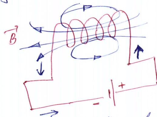
An inductor is a circuit device, usually including a coil of wire, intended to have a substantial inductance.
